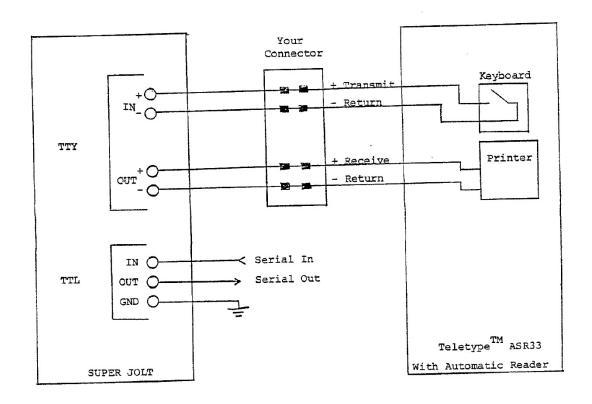
FIGURE 2. SUPER JOLT HOOKED TO A 20 ma CURRENT LOOP TELETYPE TM OR TTL INTERFACE
