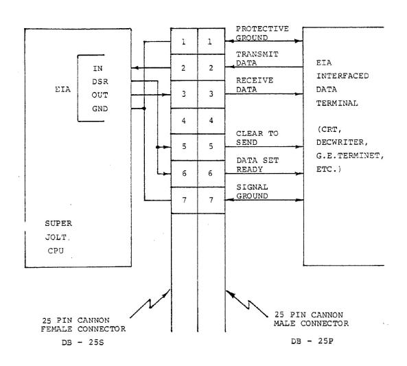
FIGURE 1. SUPER JOLT HOOKED TO AN EIA EQUIPPED TERMINAL
